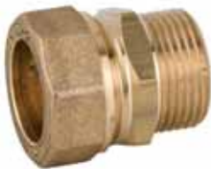
Cooper pipe fitting Brass construction. Copper pipe connection with compression ring. Male thread with flat seat for corrugated s/s. pipe.
